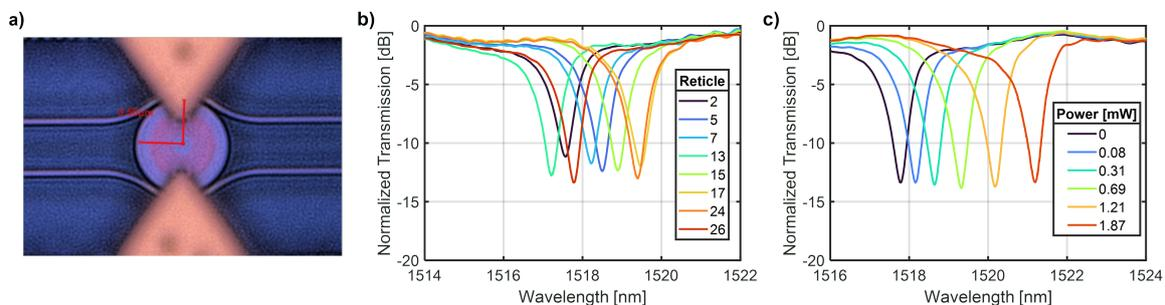
Fig. 1. **a)** Micrograph of a microdisk filter with radial couplers showing doped silicon heater geometry in redder ring at center. Bright red lines indicate scale. **b)** Transmission spectra of microdisk filters across 8 reticles. **c)** Optical sweeps of one particular microdisk device at varying heater powers.
