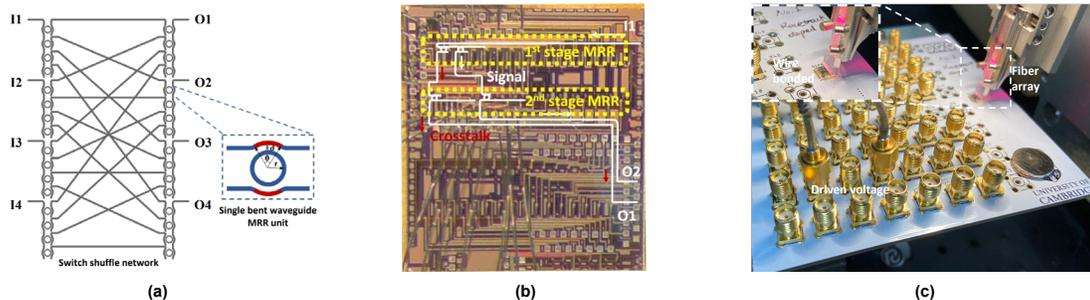
Fig 1(a) Schematic of 4×4 MRR based switch-and-select switch with bent couplers. (b) Microscope photo of the fabricated device. (c) Testbed of the silicon chip bonded onto a PCB and coupled using a fiber array.
