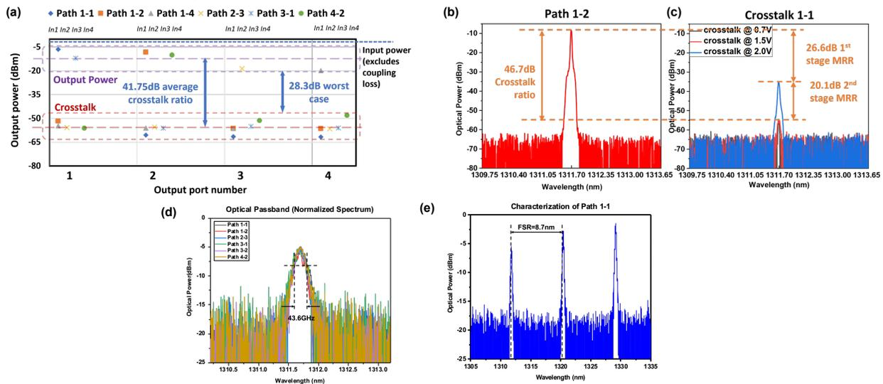
Fig 2(a) Measured optical power map of the switch, the purple and red rectangle outlines the outpower power level and crosstalk leakage, respectively. (b) Overall crosstalk ratio measurement for path 1-2. (c) Crosstalk leakage at output 1. (d) Normalized spectra of a set of representative paths, resolution is set at 0.02nm. (e) Free-spectral range of the MRR switch.
