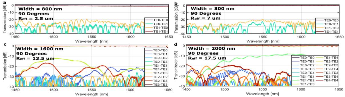
Fig. 3. Measured per-bend modal-spectral transmission of 220 nm x Width waveguide Euler bends, for 90° bends with **a)** Width = 800 nm,  $R_{eff} = 2.5 \mu\text{m}$ , and modal crosstalk  $\leq -20$  dB, **b)** Width = 800 nm,  $R_{eff} = 7 \mu\text{m}$ , and modal crosstalk  $\leq -20$  dB, **c)** Width = 1600 nm,  $R_{eff} = 13.5 \mu\text{m}$ , and modal crosstalk  $\leq -12$  dB, and **d)** Width = 2000 nm,  $R_{eff} = 17.5 \mu\text{m}$ , and modal crosstalk  $\leq -10$  dB.
